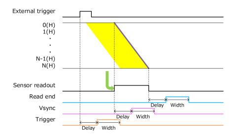
Figure 11-22 Programmable timing output (Top to bottom readout)
