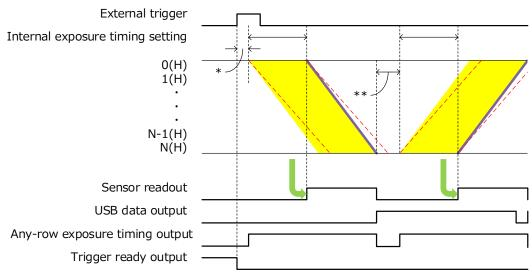
\* Delay: 42H(16bit), 36H(12bit), Jitter:  $\leq$  1H \*\* Blanking time : Minimum 78H(Depends on amount of transfer data) 1H readout time : 12.19  $\mu$ s - 320  $\mu$ s(16bit) 5.167  $\mu$ s - 320  $\mu$ s(12bit)
