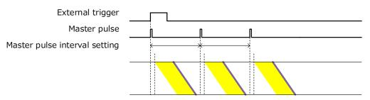
Figure 11-26 (Camera: Normal area, Edge trigger mode) (The number of pulses is specified as 3)
