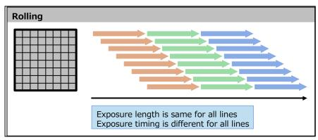
Figure 10-2 Readout timing of Rolling shutter
