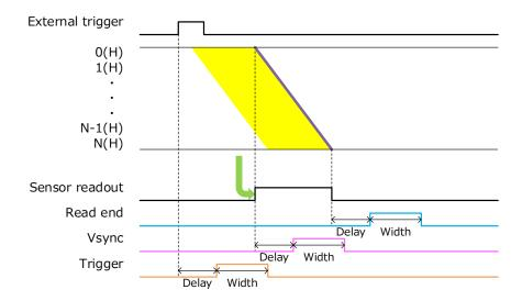
Figure 11-11 Programmable timing output
