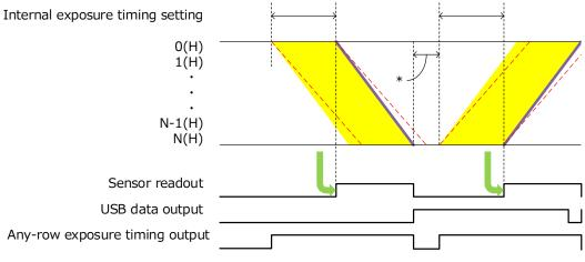
\* Blanking time : Minimum 78H(Depends on amount of transfer data) 1H readout time : 12.19  $\mu$ s – 320  $\mu$ s(16bit) 5.167  $\mu$ s – 320  $\mu$ s(12bit)
