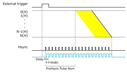
Figure 11-23 Programmable timing output referenced with Hsync (Top to bottom readout)
