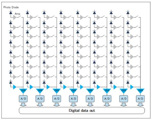
Figure 10-1 Structure of CMOS image sensor
