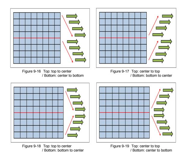
W-VIEW Mode supports Binning readout, Sub-array readout and Rapid rolling mode. In sub-array mode, the vertical position of sub-array readout can be set independently in the top and bottom areas.
