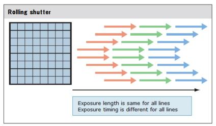
Figure 9-2 Exposure timing of Rolling shutter
