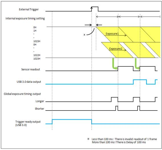
Figure 9-22 (Start trigger mode)
