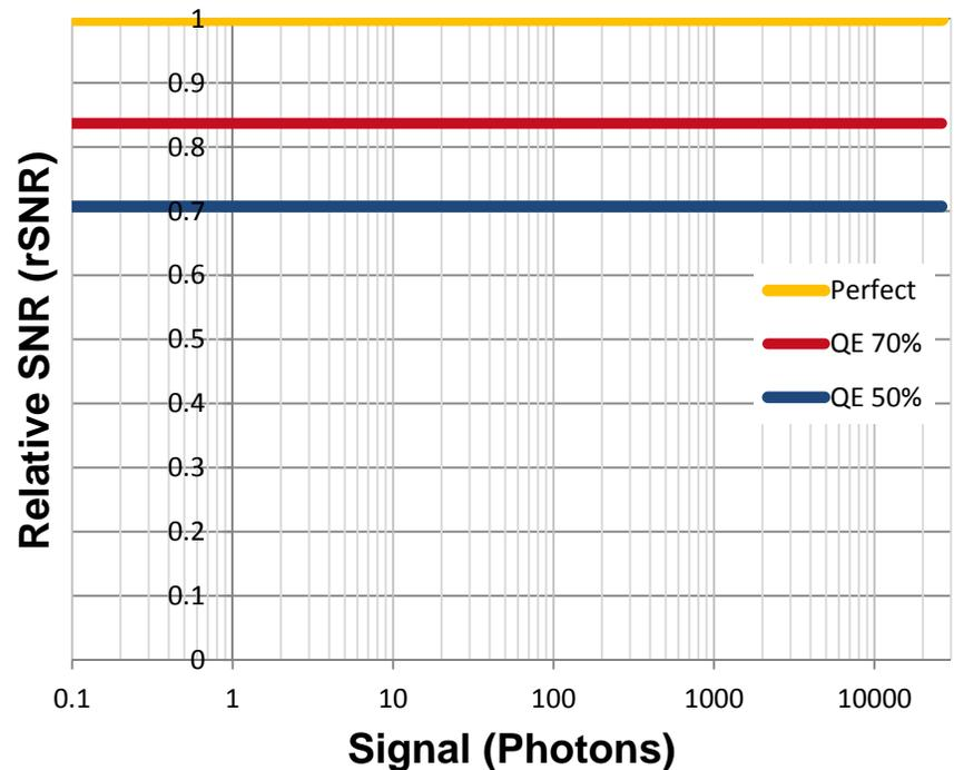
rSNR is the SNR for a camera plotted relative to the perfect camera
