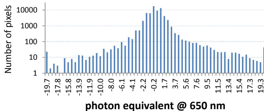
Does not fit a Gaussian distribution, i.e. is not completely modeled by a single "read noise."
