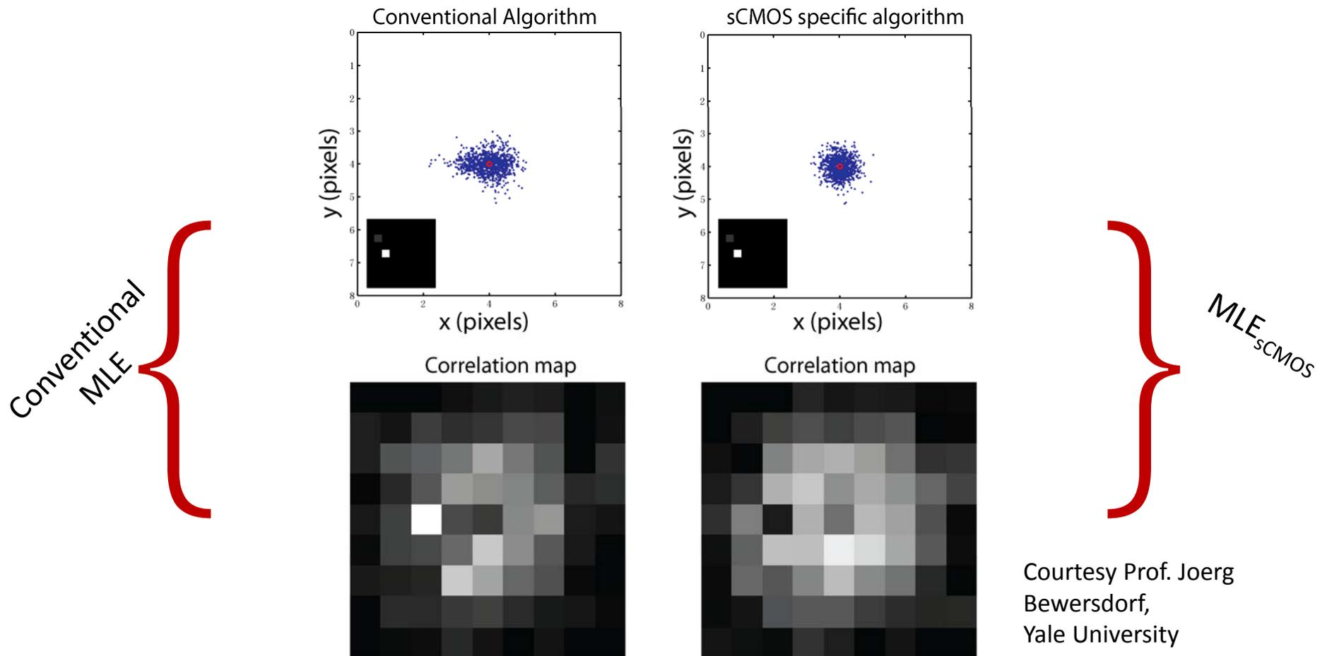
Incorporating pixel-specific read noise into the Maximum Likelihood Probability Model eliminates and narrows the asymmetric distribution of localized molecules caused by higher read noise pixels.
