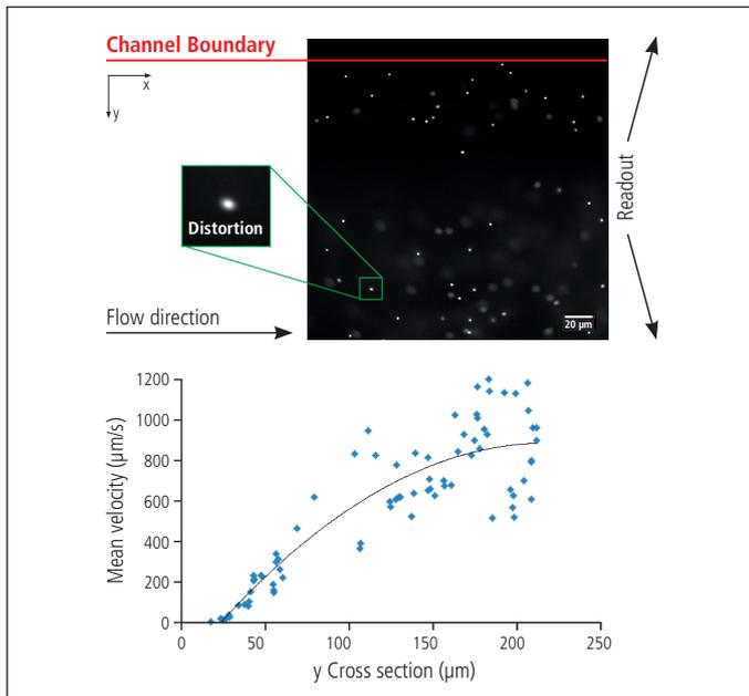
**Fig. 2: (top) Snapshot of 1  $\mu\text{m}$  latex beads recorded at full width of view (2048 x 2048 pixels or 211 x 211  $\mu\text{m}$ ). (bottom) Average velocity of the particle tracks along the y cross section of the channel.**
