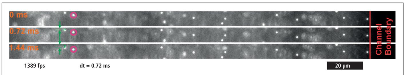
**Fig. 3: Time stack of sub-array video using "light-sheet" image acquisition. The exposure time is 9.74  $\mu\text{s}$  and the frame rate is 1389 fps ( $\text{fps}=1/(\text{80 pixels} \times 9.74 \mu\text{s})$ ). The purple circle indicates a micro-bead at 1000  $\mu\text{m/s}$  and the green marks shows the distance the bead traveled during image acquisition.**
