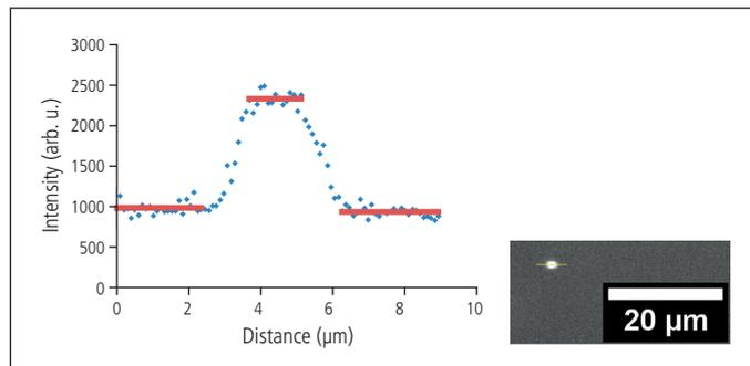
**Fig. 1: Line intensity profile of a poly-fluorescent microsphere using a standard eGFP filter set. Even at bright background signals the sample signal is very high yielding a signal-to-background ratio of 2.4.**
